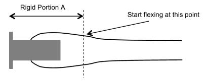
d. In an effort to assist customers with the correct installation of a dock hose, Novaflex has listed suggested support areas that incorporate the bend radius of the hose. It is common to build a curved support to prevent over bending at the coupling area.
